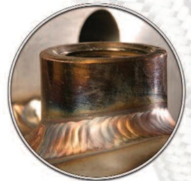
This Flextrol fitting illustrates our high quality fabrication and welding. The light rainbow effect is the result of correct, even heating during welding. Overheating can weaken the metal, leading to failure of a fitting, joint, or hose.
